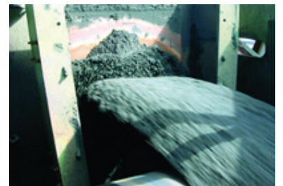
KERAFLEX installed at a ship unloading facility handling taconite.
