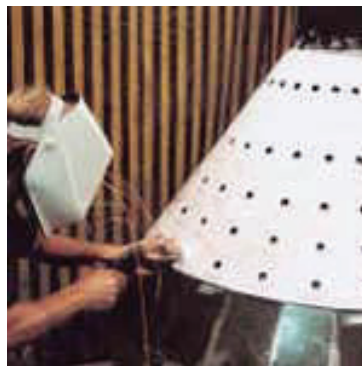
Weld-on KALOCER® high alumina ceramic tiles protect this cone against wear and thermal shock.
