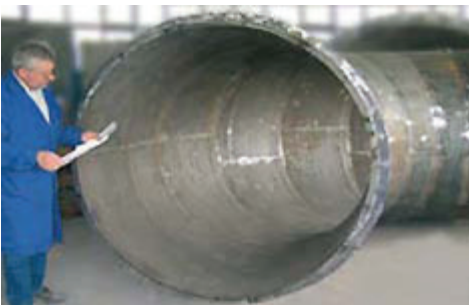
Clinker dust pipe: cyclone exit protected with KALMETALL® W.
