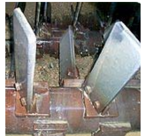
Paddles made of KALMETALL-C 153 installed in a gravel washing unit.
