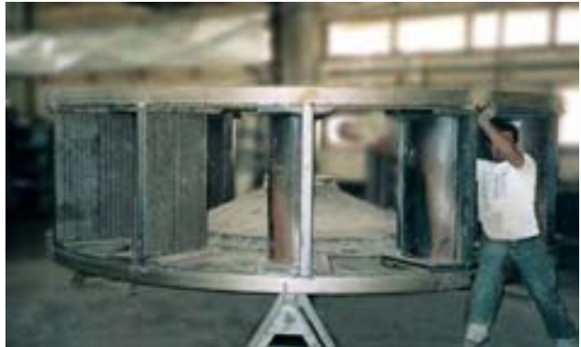
Impact coal pulverizers operate in lignite fired power plants; the impact plates have been lined with KALMETALL-W 100
