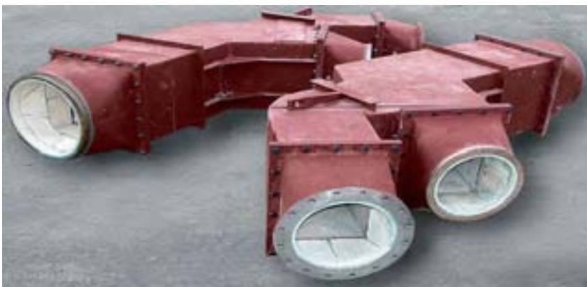
PF-distribution boxes protected with KALCOR for large area lining and KALOCER to ensure maximum wear resistance
