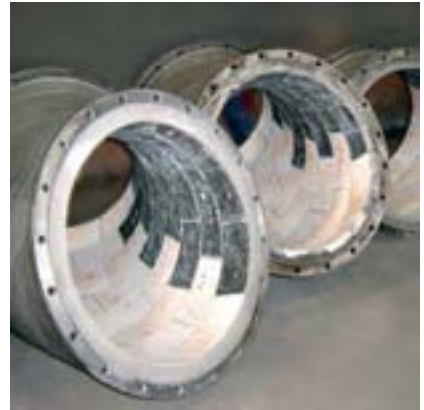
Material combinations of KALCOR and ABRESIST provide economic wear solutions
