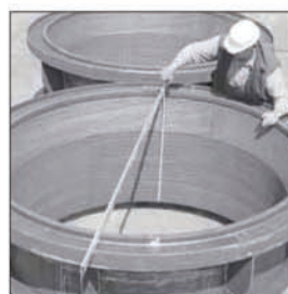
Separating cones of cement classifiers made of KALMETALL-W 100 6+4, 3,000 mm diameter
